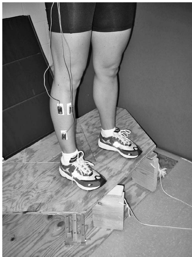
Figure 2. Experimental setup and electrode placement for the peroneus longus, peroneus brevis, and tibialis anterior muscles.
