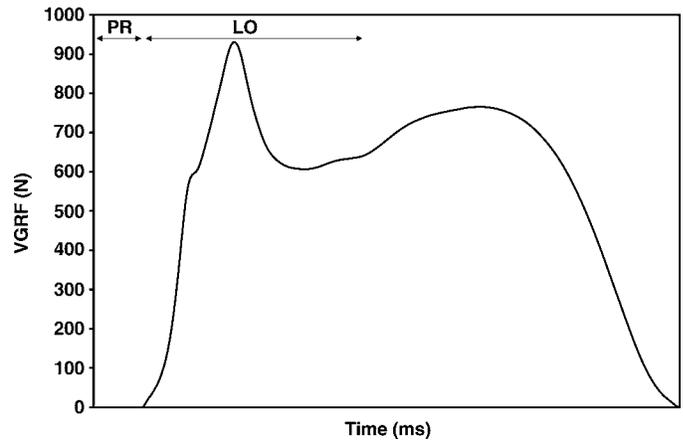
**Figure 3.** Preparatory phase (PR) was defined as the 50-ms time period before vertical ground reaction force rises above 5 N. The loading phase (LO) was defined as the first 50% of the stance phase during the side-step cutting tasks.
