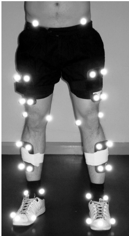
Figure 1. Positions of markers used to define the position and orientation in space of the body segments.
