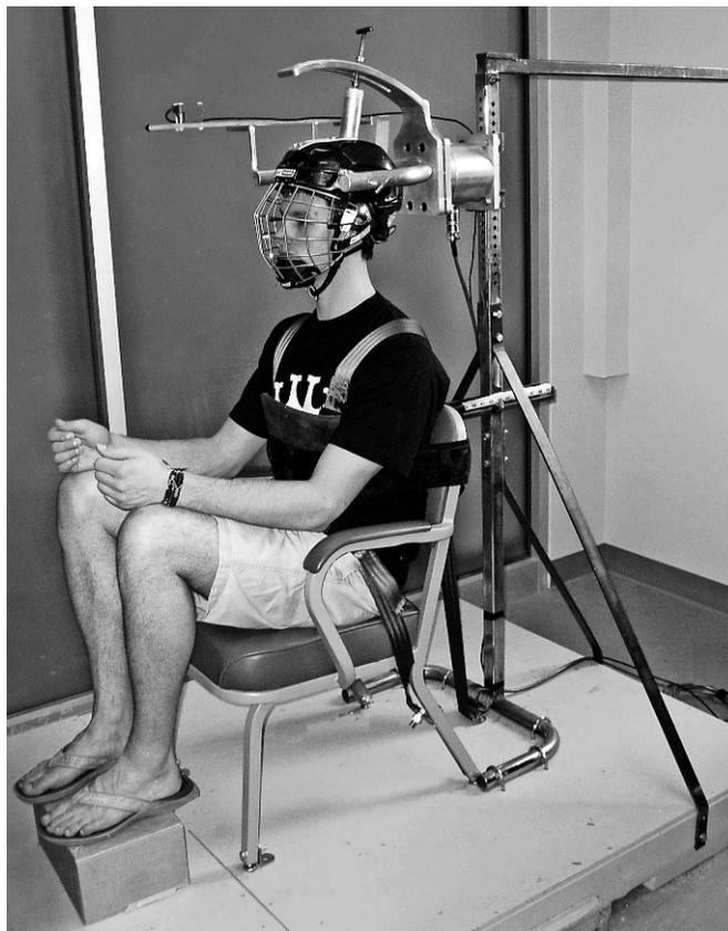
**Figure 1. Standardized position of the participant in the neck strength testing device. Adapted from Almosnino S, Pelland L, Pedlow SV, Stevenson JM. Between-day reliability of electromechanical delay of selected neck muscles during performance of maximal isometric efforts. *Sports Med Arthrosc Rehabil Ther Technol.* 2009;1:22. doi:10.1186/1758-2555-1-22. Published September 23, 2009. BioMed Central Ltd, London, United Kingdom.**
