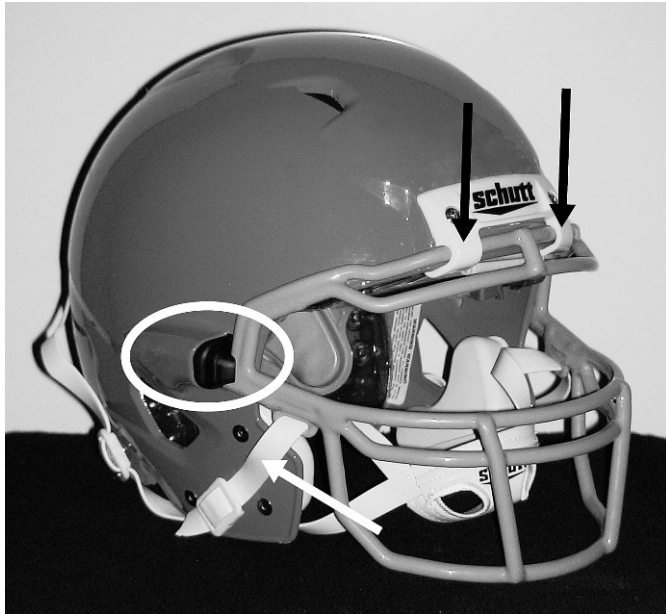
Figure 6. The ION 4D (Schutt Sports Inc, Litchfield, IL) helmet. The black arrows point to the locations on the face-mask retainer clip that need to be cut. The white arrow indicates the approximate location where the chin strap needs to be cut on both sides. The face mask inserts into the channels on each side of the helmet (white circle) and slides out when the chin straps and retainer clip are cut.
