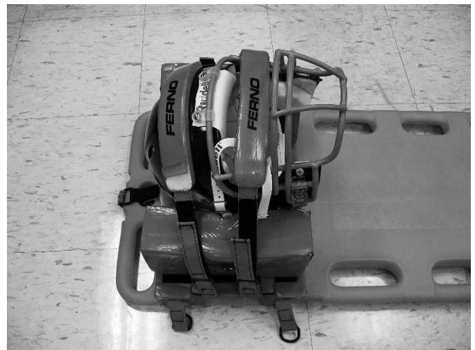
Figure 3. Helmet secured to a spine board (Ferno-Washington, Inc, Wilmington, OH) with foam blocks and straps for the testing procedure.
