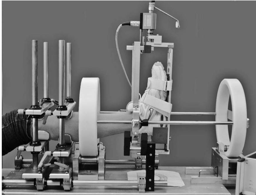
**Figure 3.** Apparatus for the measurement of maximal joint angles in 3 movement planes (6 directions) with an induced torque of 9 and 12 Nm only for dorsiflexion. Here, the unbraced condition is illustrated.
