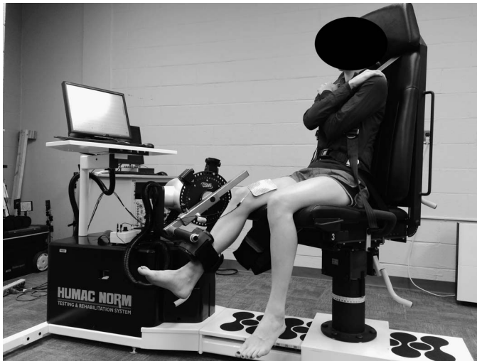
Figure 1. Participant position for maximal voluntary isometric contraction.
