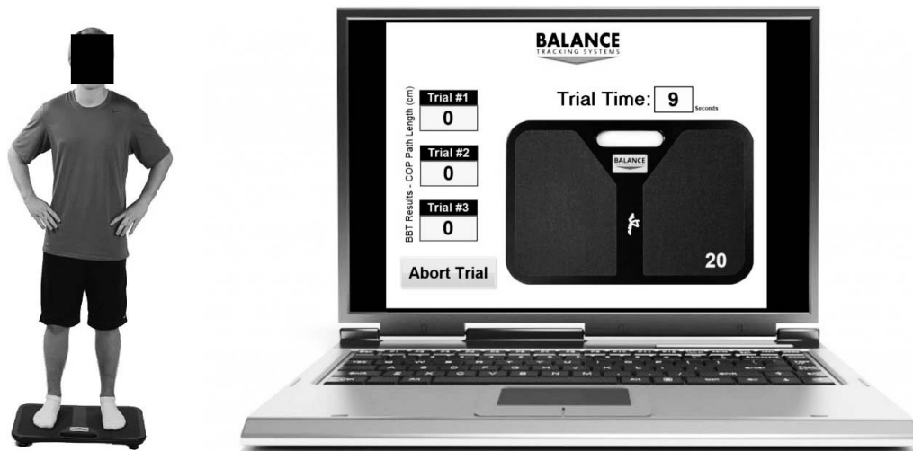
Figure 1. Depiction of the BTrackS Balance Test testing setup. Athletes stood as on the left with eyes closed, hands on hips, and 2 feet on the BTrackS Balance Plate (Balance Tracking Systems, Inc, San Diego, CA). During testing, the BTrackS Sport Balance software shown on the right guided the tester through measurement of center-of-pressure path length. In this screen shot, the first of 3 trials is in progress with a center-of-pressure path length of 20 shown on the BTrackS Balance Plate image.
