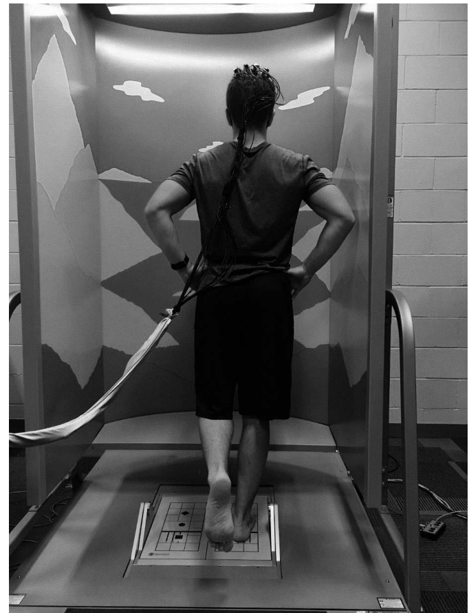
Figure 1. Testing setup on the force platform (Balance Master System 8.4; NeuroCom, Clackamas, OR) with the functional near-infrared spectroscopy system affixed to the head.
