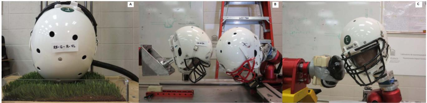
**Figure 1.** Reconstruction setups for each type of event. **A,** Fall. **B,** Helmet-to-helmet collision. **C,** Shoulder-to-helmet collision.
