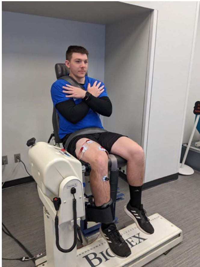
Figure 1. Maximal voluntary isometric contraction testing position using an electromechanical dynamometer.
